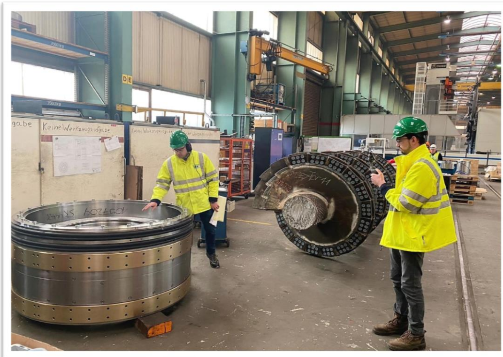
Internal Components of HRBT TBM (including screw conveyor for transporting excavated soil)
