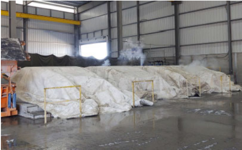
◀ Precast Tunnel Segment Liners Steam cure of cast elements
