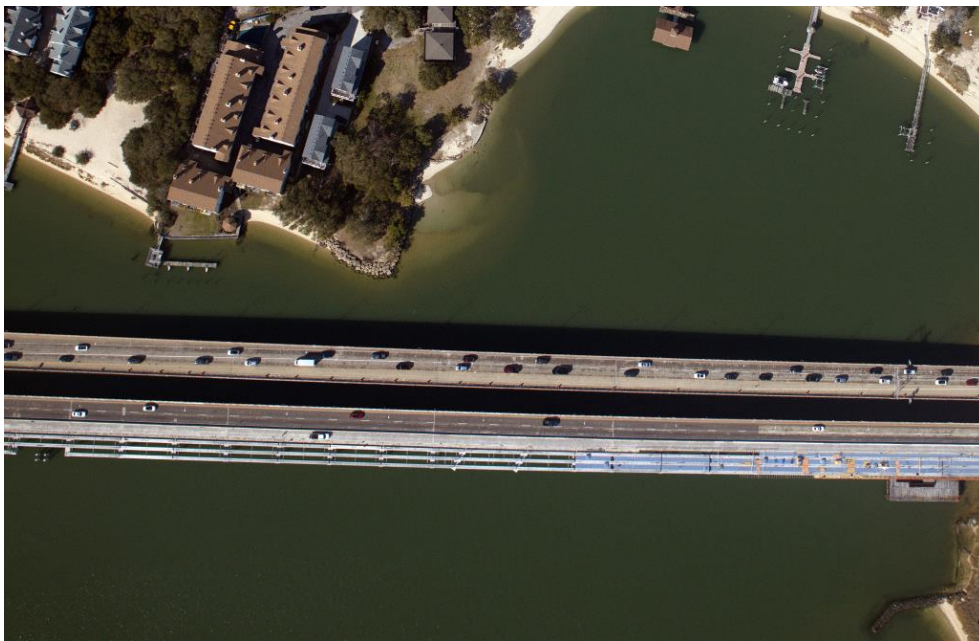
◀ Willoughby Bay Bridge Preparations for deck concrete placement at widening of eastbound existing bridge
